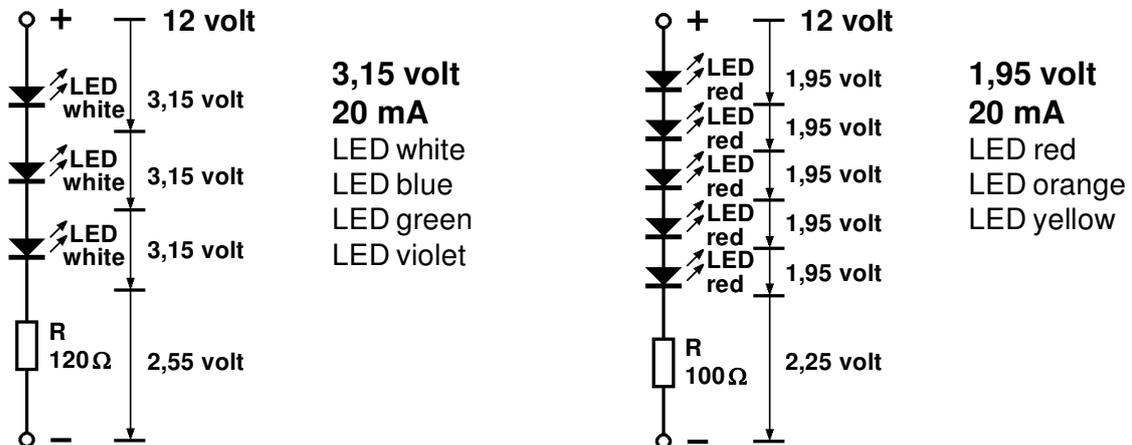
If you have a power supply with **12 volt**, it is not possible to have more than 3 white (blue, green, violet) LEDs in a row or more than 5 red (orange, yellow) LEDs in a row.
